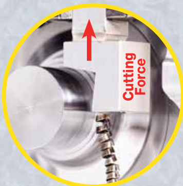
Excellent Chip Evacuation and Stable Machining
