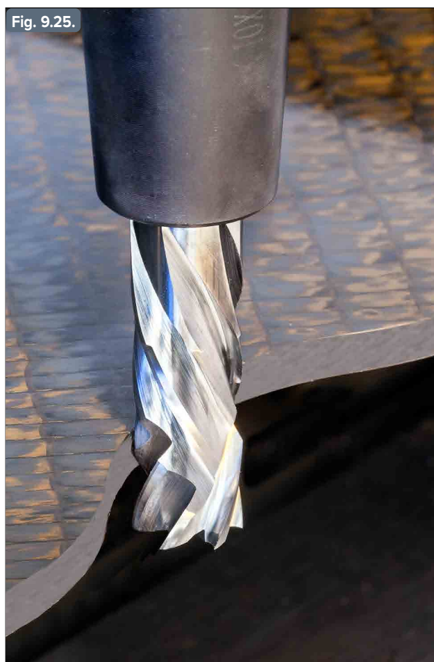
Fig. 9.25. Solid carbide endmill with right- and left-hand helix for machining composite materials
