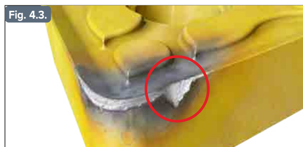
Local flank (notch) wear
