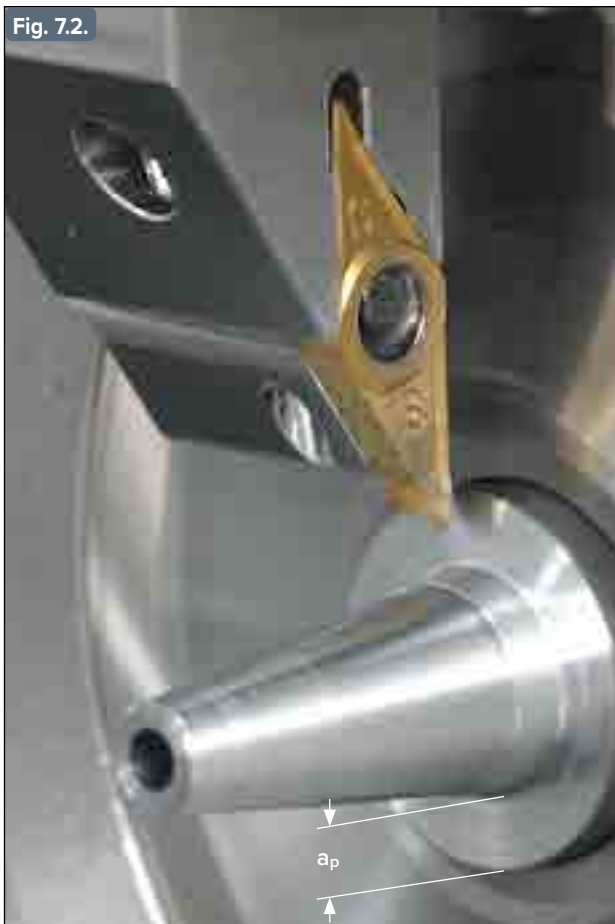
Depth of cut in turning
