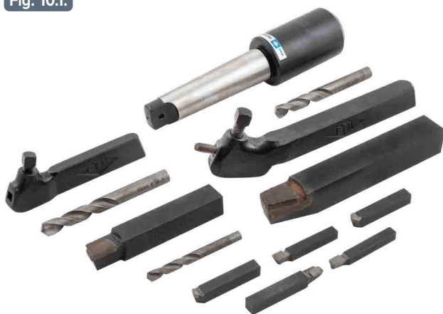
Typical brazed tools. These tools prevailed in the carbide tool design for a long time.
