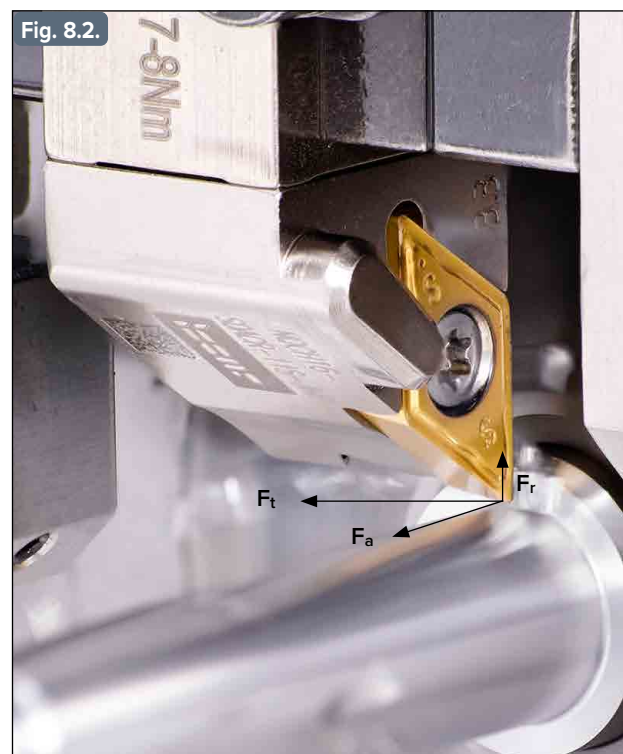
Fig. 8.2. Cutting forces in turning
