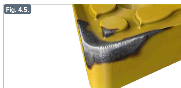
Chipping of the cutting edge
