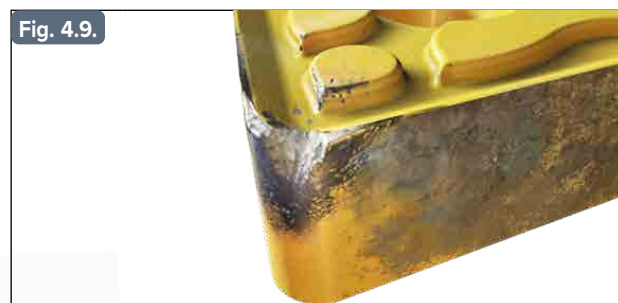
Catastrophic failure (fracture) of cutting edge
