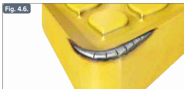
Comb cracks
