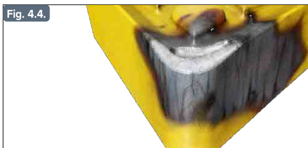
Face wear in the form of crater wear
