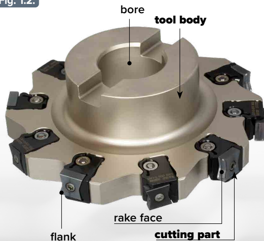
a milling tool (rotating, multi-point, assembled, bore-type, adjustable)
