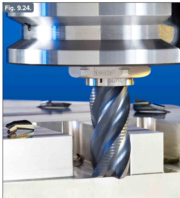
FINISHRED "two-in-one" endmill
