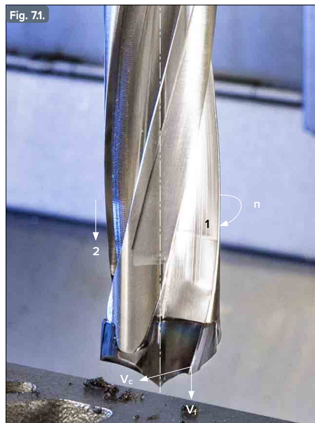
Motions and motion velocities in drilling.
